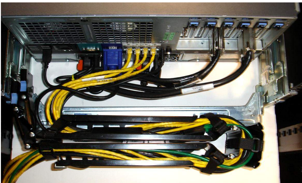
Figure 12. T710 CMA Mounted on the Left Side
