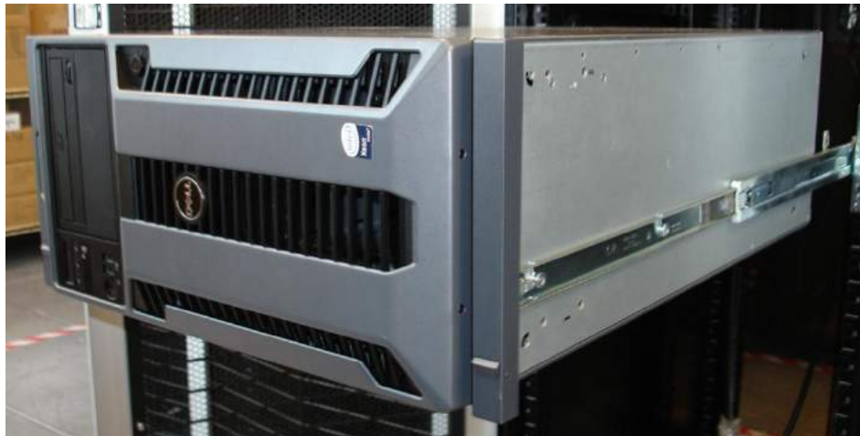
Figure 11. T710 Mounted in the C1 Sliding Rails
