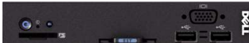
Figure 7. Rack system with VGA port
