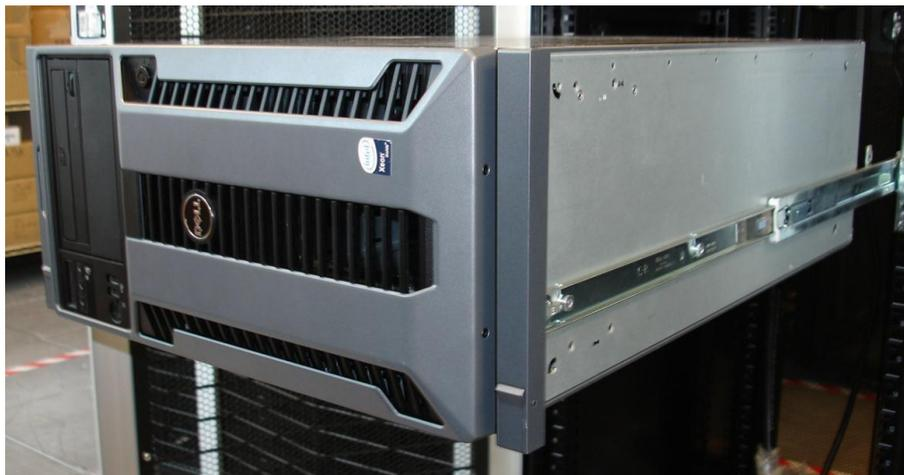
Figure 12. T610 Mounted in C1 Sliding Rails
