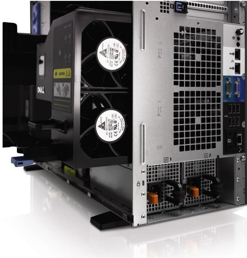
Figure 5. Fans and Cooling Shroud
