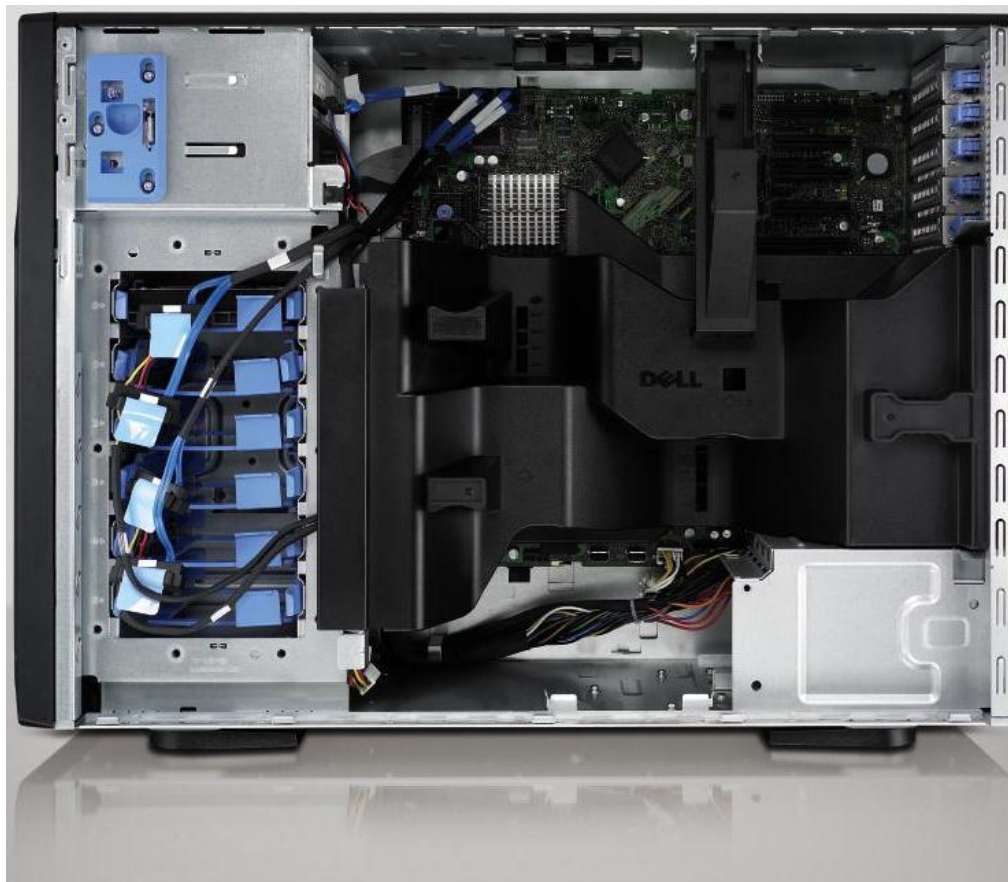
Figure 7. Internal View (Cabled Hard Drive Configuration)
