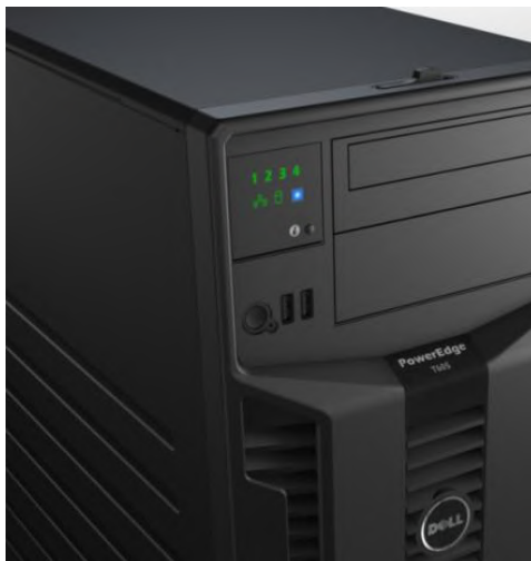
Figure 10. LED Control Panel
