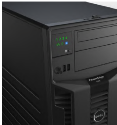
Figure 5. LED Control Panel
