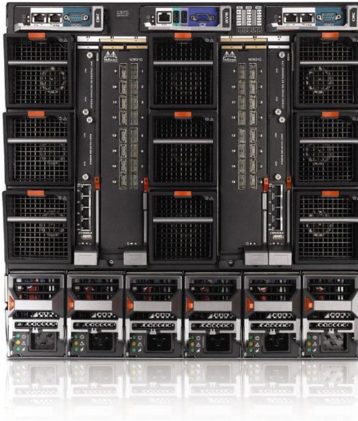
Figure 10. Rear View Showing Fans
