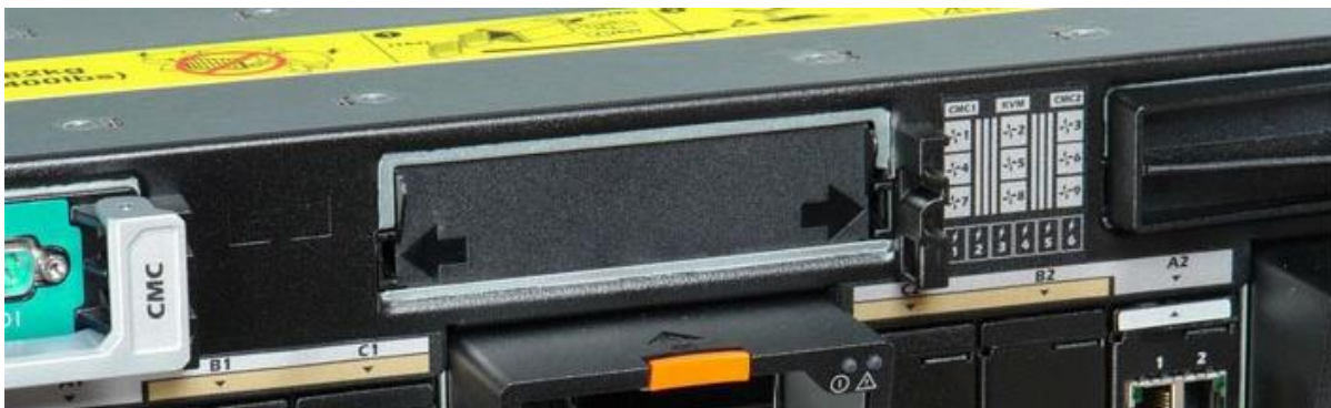
Figure 15. Installed iKVM Blank
