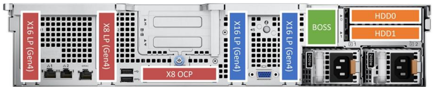
Figure 12. Rear view of the system with no riser and two CPUs
