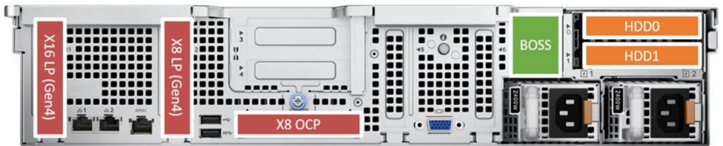
Figure 11. Rear view of the system with no riser and one CPU
