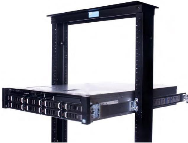
Figure 25. Static rails in 2-post center mount configuration
