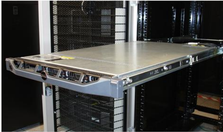
Figure 11. R610 Mounted in the A1 Sliding Rails
