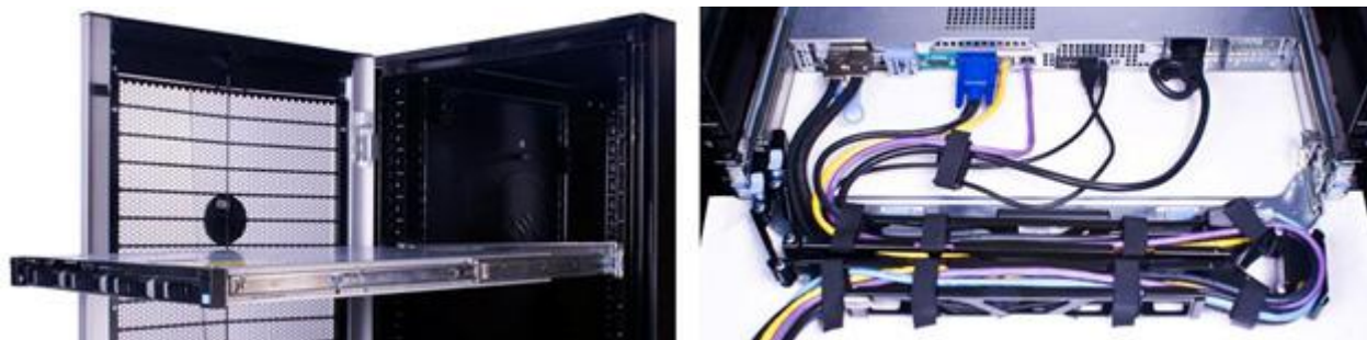
Figure 18. System mounted in sliding rails with the CMA
