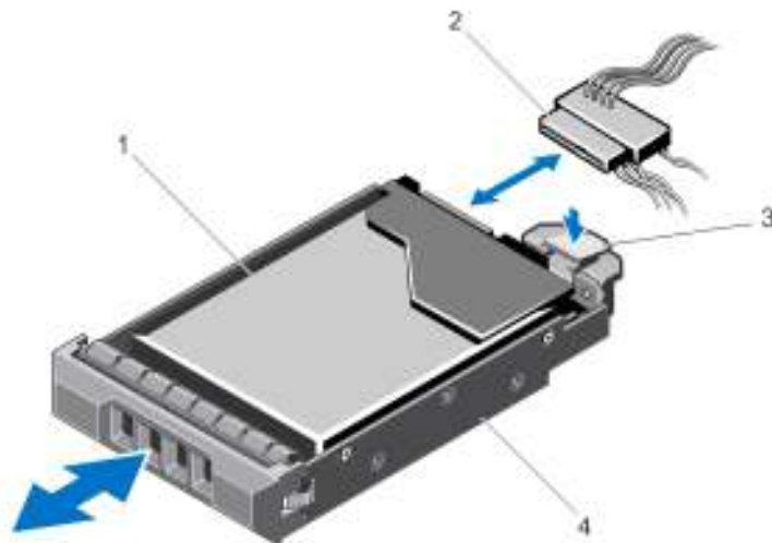
Figure 22. Removing and Installing a Cabled Hard Drive
